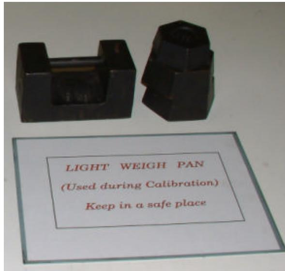
Place the light weigh pan squarely on the weigh pan with the balance locked position as shown.
