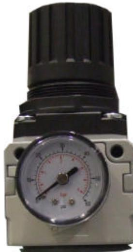
Check the air to the dispense and re-circulate valves is set correctly. This is set by means of the regulator mounted on the side of the control box. This is set to 5.5bar at the factory and is the recommended pressure.
