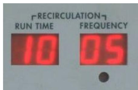
The timer is started when run mode is entered (from set mode). The next recirculation will start at the same time every hour, two hours, etc. at the time value which was entered. The timer will reset if set entered and then run mode is re-entered.
