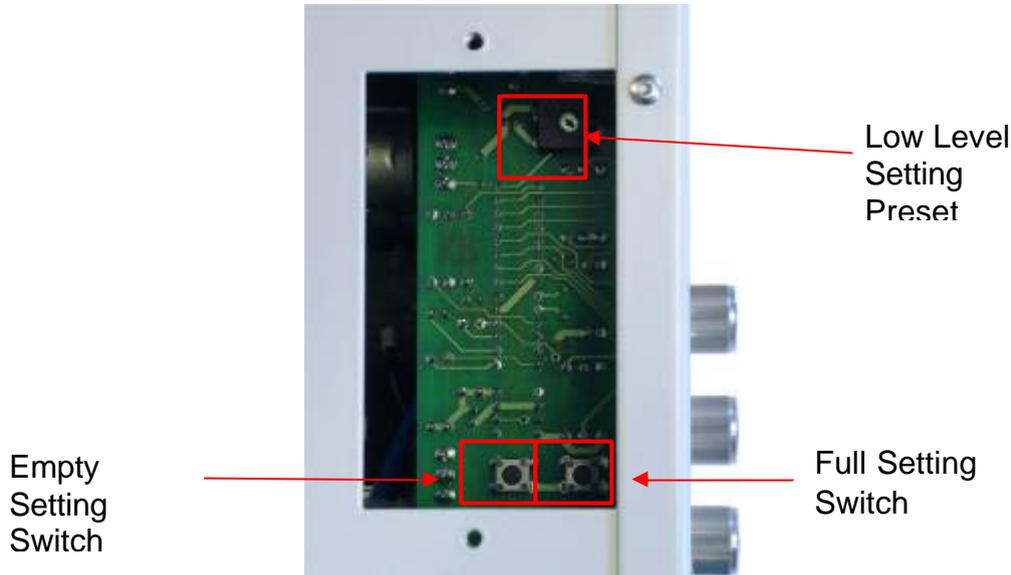
Remove the lid from a full drum of product to be dispensed through the drum dispenser. Insert the level sensing probe (mounted on the ink supply hose) into the product to a depth of 20mm and press the empty setting switch shown above which will set the empty point.
