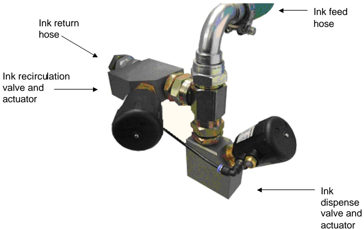
The recirculation valve comprises a valve body and an actuator which is also controlled by the LA Control Unit. It will open as determined by the setting of the control unit. As the actuator is activated, the restrictor in the valve body is opened and the ink is pumped through the return hose and back into the drum.
