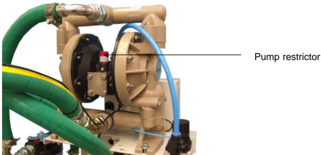
In the centre of the restrictor is a socket head bolt or slotted adjuster. Turn this bolt anti-clockwise (upwards) to de-restrict the pump, stop when the bolt comes into contact with limiter pin. This will allow free flow of ink through the pump, and can be adjusted if necessary when the pump has been primed with ink.
