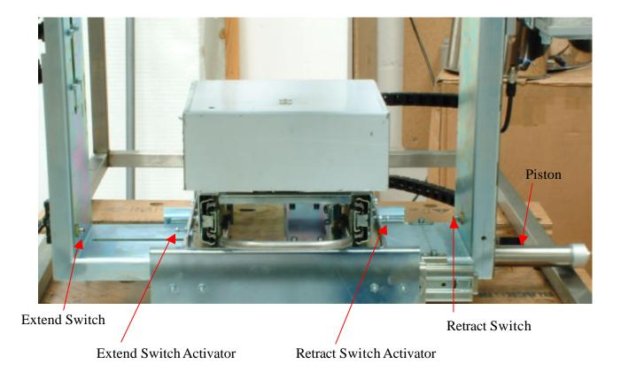
The balance is moved from Left (Extend) to Right (Retract) by the Air Piston.
