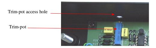
Using a flat blade terminal screwdriver, (0.5X3X60 for example) adjust the trim-pot to give the required reading of 3000. (The light-weight pan should be on while making the adjustment and the rest of the calibration procedure). Follow the on screen prompts to complete the calibration.
