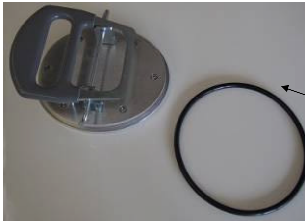
Ink Supply Container lid with gasket removed
