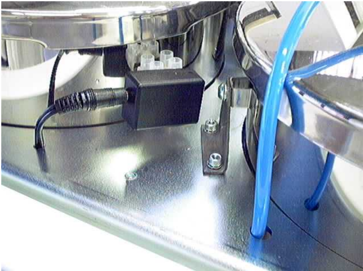
Figure 4. Correctly mounted Jack Plug and Digitizer
