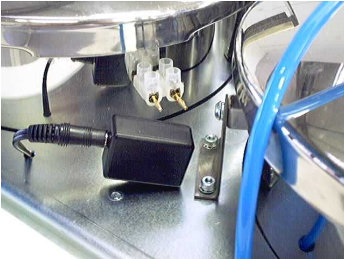
Figure 1. Digitizer and Jack Plug fallen off reservoir (Usually found after rough transportation of the IDS)
