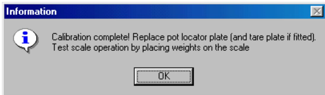
The Calibration is now complete; please replace the Pot Locator Plate (and Tare Plate if fitted)
