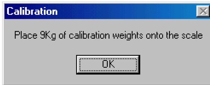
Place 9Kg (5Kg,2Kg,2Kg and 1Kg) Weights onto the Balance/Scale
