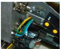
Route the 1260mm Earth Strap under the Scale Box, behind the
