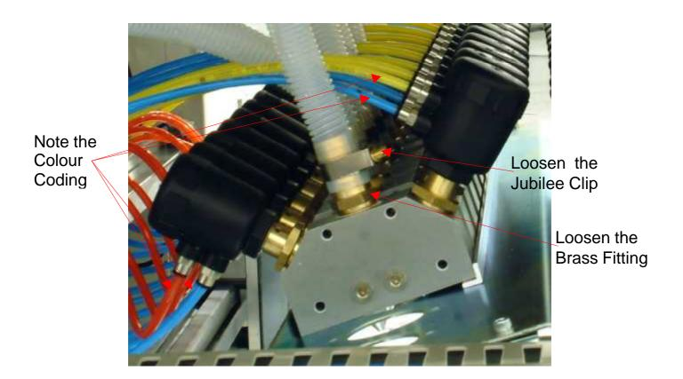
Remove the air pipe, push the black collar on the air fitting in and then pull the pipe out while holding the collar in. Loosen the Brass fitting but do not remove it at this stage.
