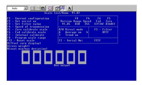
Place weights to the FSD - 10% on the weigh pan, (e.g. 27kg for a 30kg scale range), allow the scale to stabilise for a couple of minutes and press the FSD function key 'F6'. The displayed value will change and the message 'Calibrating' will appear below it. The number will count up for about three to four minutes, after this time the 'Calibrating' message will change to 'Hex reading'. Calibration can also be done showing the weight as shown.
