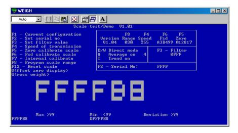
Remove all weights and place the pot locator plate on to the weigh pan, press the 'W' key so that the scale is displaying weight, and press the 'O' key to 'Offset' the reading to zero.
