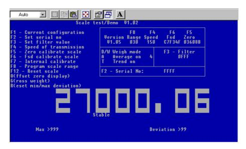
During the calibration process the speed of the boards data transmission will have been slowed down, this should be set back to 255 using the 'Speed' function key F4. Press F4, enter 255, then hit return; the value of 255 will replace 150 under the 'Speed' heading.
