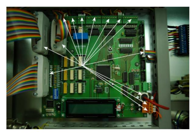
5. Now undo all the mounting screws from the controller
