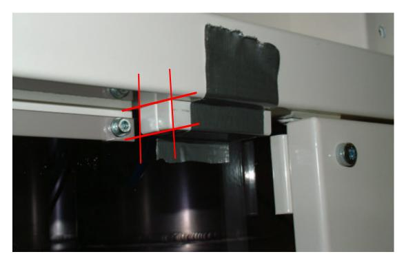
Attaching the magnet as shown will allow the Dispenser to be operated with the door open for diagnostics and fault finding and door switch alignment issues.
