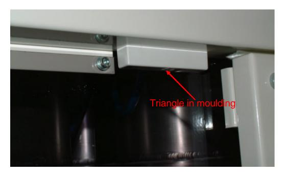
Using the small triangles in the mouldings, align the magnet assembly to the reed switch assembly as if the door was closed, it is important that they are flush as shown:
