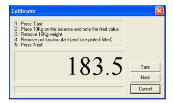
The screen shown above is the scale calibration screen showing current weight and instructions on creating pre-calibration figures, if it has been established that the scale is out of calibration and the figures have been recorded, this part really isn't required. If calibration is not required, cancellation of the procedure can be achieved at this point. Clicking on next will start the calibration procedure which is irreversible.
