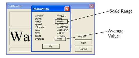
This is the basic scale programming information stored on the Scale board that we may ask for if you are having trouble calibrating the scale, check the Scale Range is correct; the example above shows a 10Kg range Scale Board. The Average setting should be 02 on all scales but for the Integra Formulator Scale which is set to 04.
