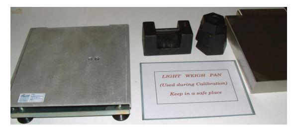
Place the Light Weigh Pan/Calibration Plate squarely on the Internal Weigh Pan as shown below:
