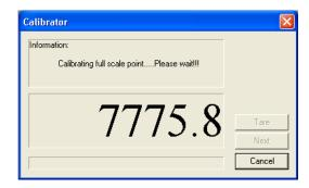
The final value, in this case 9Kg will be displayed as the value is stored, during the last stages it is again important that the scale is not exposed to vibrations drafts or touched during this period.
