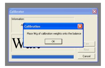
Place 9Kg of conformance or Calibration weights centrally on the scale stacked with the Balance Retracted and Locked as shown below:
