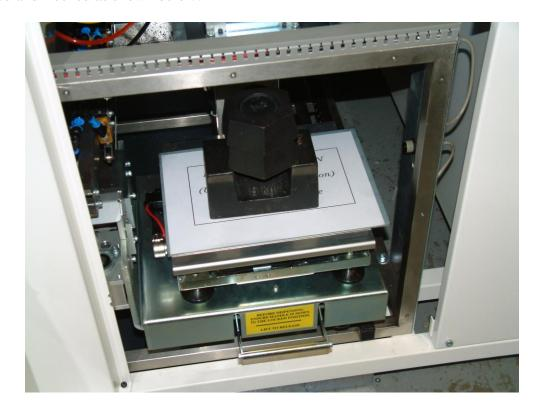
Click OK, the scale will then allow time for the readings to settle before values are displayed counting up to the calibration weight value, this will overshoot up to three times reducing less each time as the calibration point is homed in on as shown:
