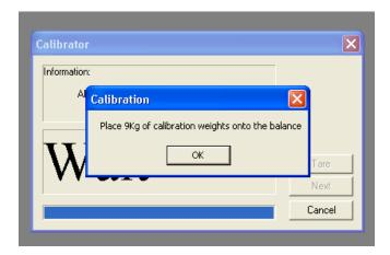
Place 9Kg of conformance or Calibration weights centrally on the scale stacked as shown below:
