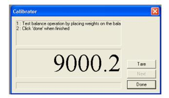
The scale calibration can be tested using this window, to do this remove all the weighs and Light Weigh Pan/Calibration Plate from the scale, replace the weigh pan and click on Tare, place the calibration weighs on the scale in 1Kg increments and record the value displayed at each point:
