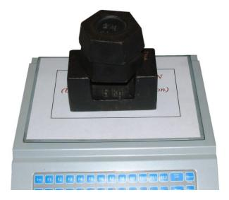
Click OK, the scale will then allow time for the readings to settle before values are displayed counting up to the calibration weight value, this will overshoot up to three times reducing less each time as the calibration point is homed in on as shown:
