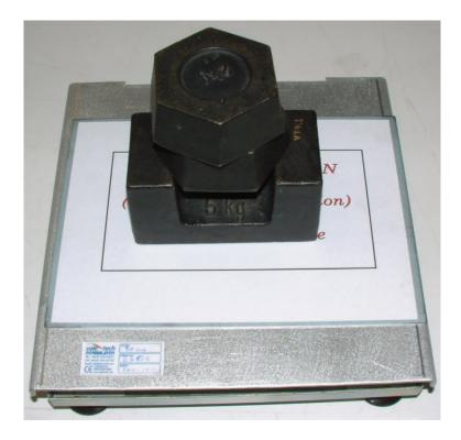
Click OK, the scale will then allow time for the readings to settle before values are displayed counting up to the calibration weight value, this will overshoot up to three times reducing less each time as the calibration point is homed in on as shown:
