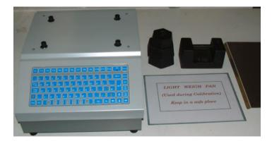
Place the Light Weigh Pan or Calibration Plate squarely on the four rubber feet which protrude through the top of the case as shown below:
