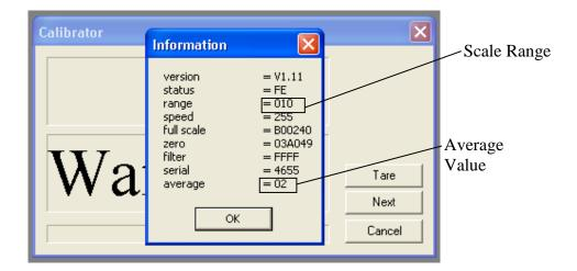
This is the basic scale programming information stored on the Scale board that we may ask for if you are having trouble calibrating the scale, check the Scale Range is correct; the example above shows a 10Kg range Scale Board. The Average setting should be 02 on all scales but for the Integra Formulator Scale which is set to 04.
