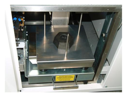
If the scale is within specification at each of the calibration points, click Done, calibration is complete. If not, click Done to close the current window and repeat the calibration procedure again. If repeating the procedure does not achieve the desired results, please contact Vale-Tech Technical Support.
