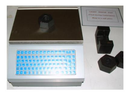
If the scale is within specification at each of the calibration points, click Done, calibration is complete. If not, click Done to close the current window and repeat the calibration procedure again. If repeating the procedure does not achieve the desired results, please contact Vale-Tech Technical Support.
