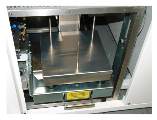
Place the calibration weighs on the scale in 1Kg increments and record the value displayed at each point, again with the Balance Retracted and Locked as shown:
