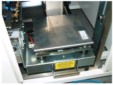
Place the Light Weigh Pan squarely on the Internal Weigh Pan/Calibration Plate with the Balance Retracted and Locked as shown below:
